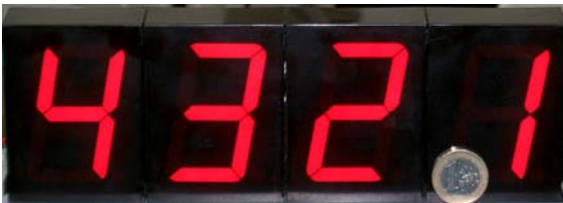
picture shows 4-spaces 7-segment display
